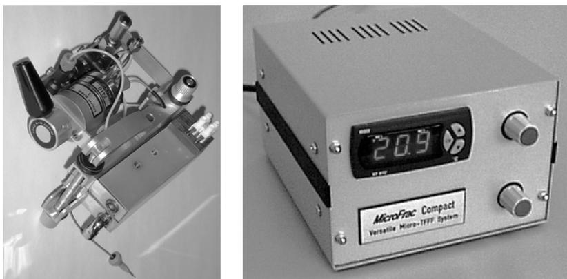
**Figure 9.** Commercial micro-TFFF versatile channel unit MicroFrac Compact and hot wall temperature controller MicroFrac.
