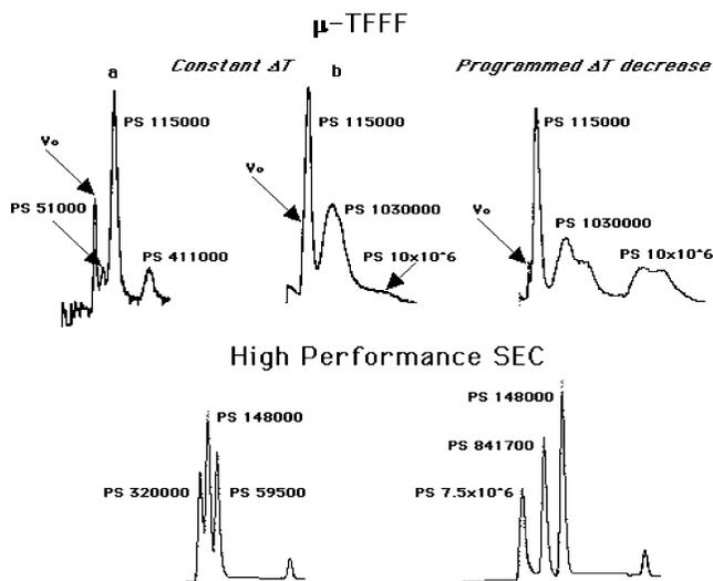
**Figure 4.** Comparison of the separations of polystyrenes carried out by micro-TFFF at constant and programmed decrease in temperature drop with the chromatograms from high-performance SEC. Reproduced with permission from Janča.<sup>[18,19]</sup>
