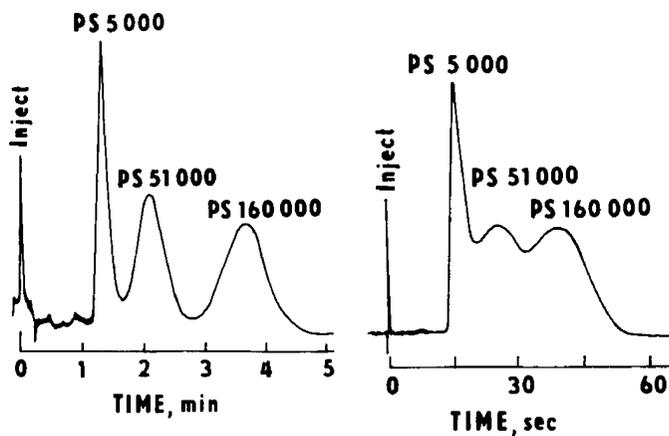
**Figure 1.** Fractograms of a mixture of three PS standards obtained at various flow rates in a TFFF channel of reduced thickness,  $w = 0.0051$  cm. Reproduced with permission from Giddings et al.<sup>[8]</sup>
