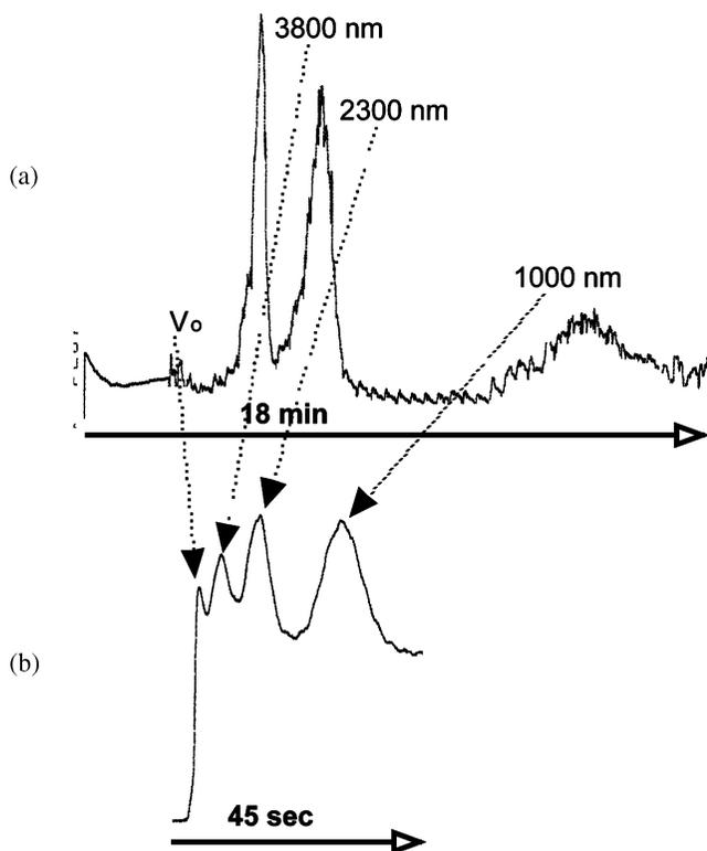
**Figure 3.** High-speed separation of a mixture of three polystyrene latexes obtained at various flow rates in micro-TFFF channel under the conditions of effective focusing mechanism. Reproduced with permission from Ananieva et al. and Janča et al.<sup>[16,17]</sup>
