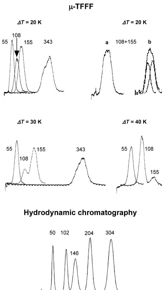
**Figure 6.** Comparison of micro-TFFF and HC applied to particle size analysis. Reproduced with permission from Janča et al.<sup>[15]</sup>
