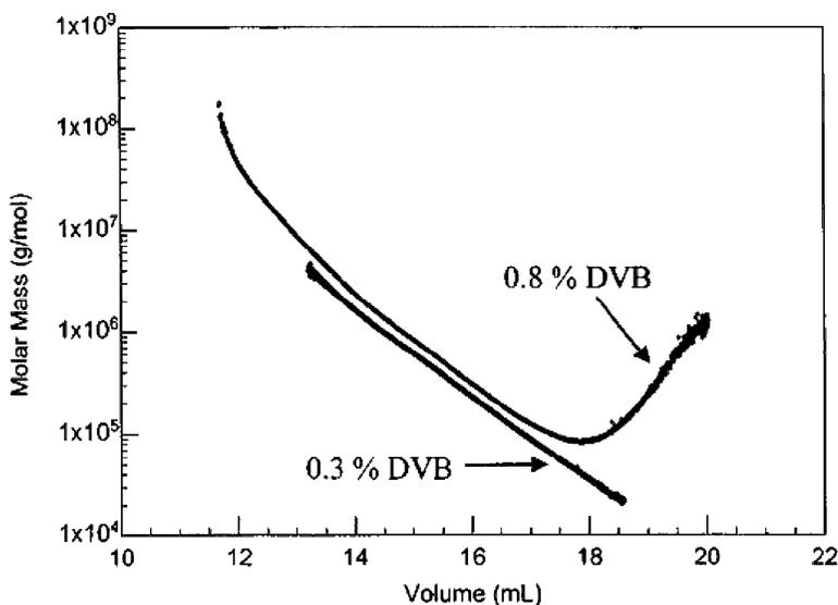
**Figure 5.** Separations of differently branched polystyrenes carried out by SEC coupled with MALS detector. Reproduced with permission from Podzimek et al.<sup>[21]</sup>
