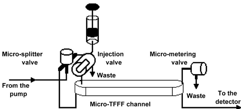
**Figure 8.** Schematic representation of the fluid circuit of the micro-TFFF channel unit.
