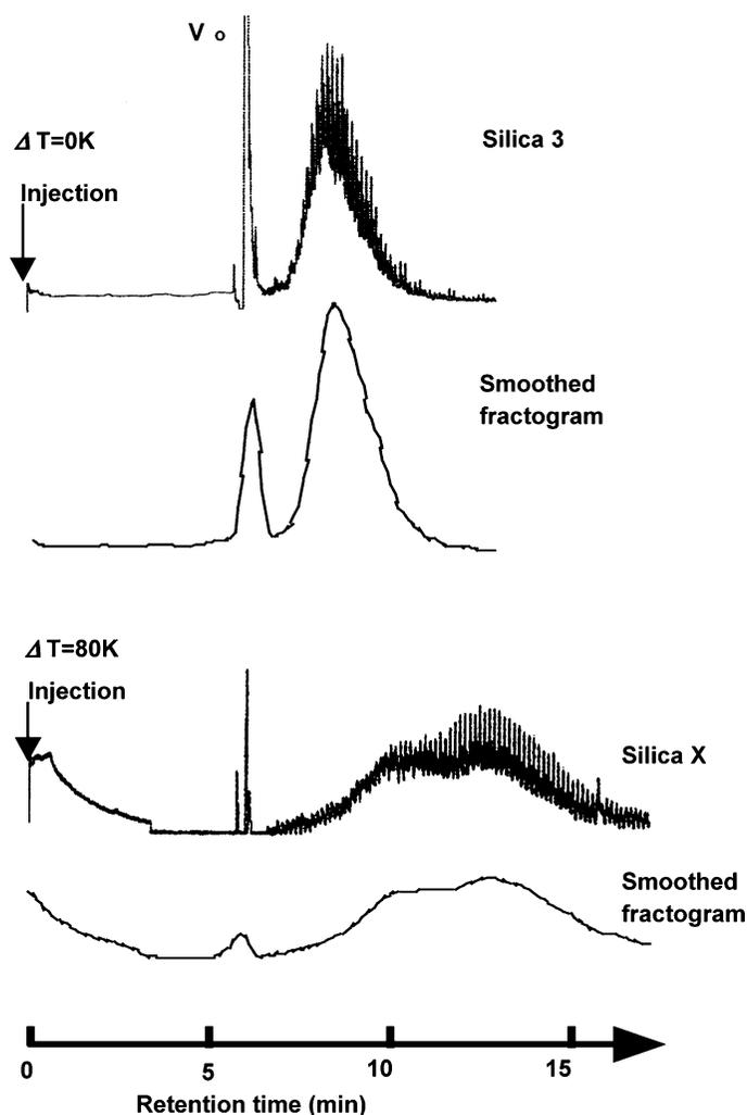
**Figure 7.** Comparison of the raw and smoothed fractograms of two silica chromatographic beads. Reproduced with permission from Ananieva et al.<sup>[29]</sup>
